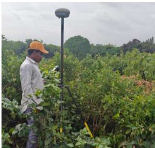
Field Photograph 10: DGPS survey at Amoch Chhapra block
