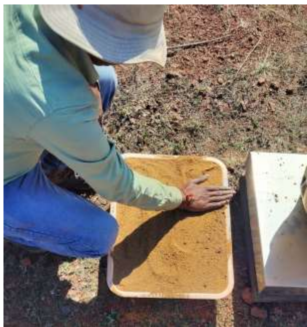
Field Photograph 15: Measurement of sand volume
