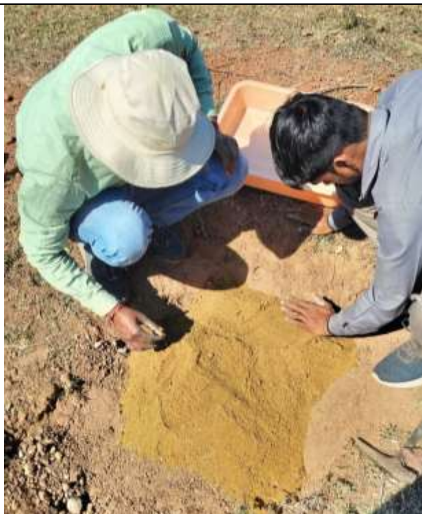
Field Photograph 16: Pit filling with sand
