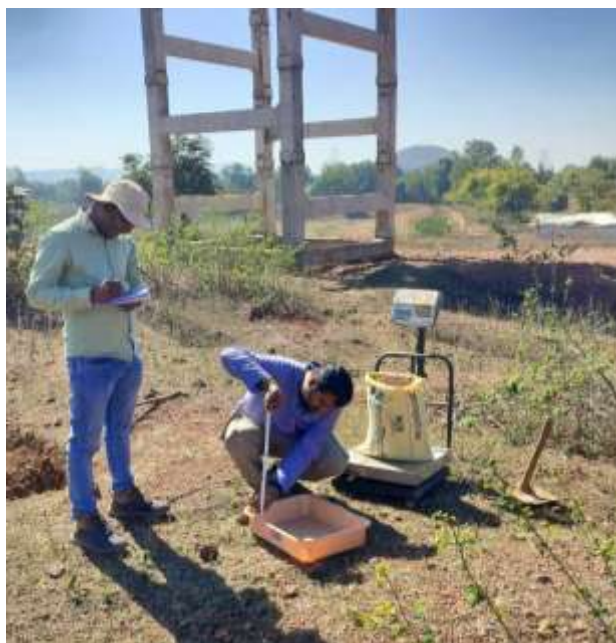
Field Photograph 14: Measurement of excavated material mass
